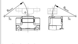
$R_{\mbox{\scriptsize Amin}}$  and  $R_{\mbox{\scriptsize Bmin}}$  depend on the actuator. Applies accordingly also to lateral retraction directions.
